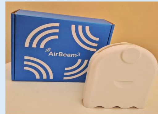
Airbeam low-cost palm sized air quality instrument Sensor in Limpopo - Lephalale
